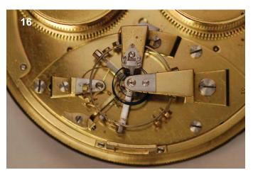
The pointed oval escapement platform (16) comprising the balance, detent, and escape wheel is fixed to the main movement plate with three screws. The balance spring stud (top showing) and its clamp are very clear in this photo. You will notice there is a protective gate screwed to the bezel to protect the balance and escapement from errant fingers and for safety when the movement is placed into the tub.
